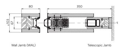
Horizontal Section Through Standard Panel (NE)
